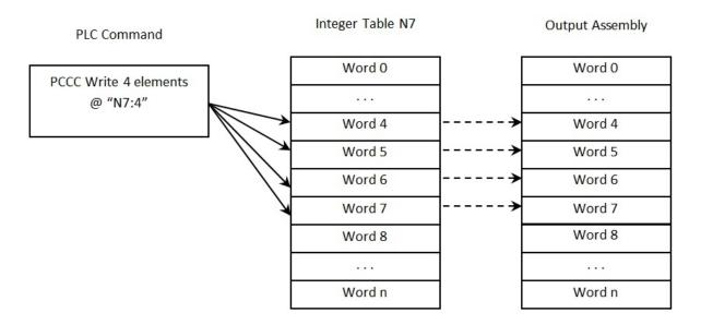
The bit to trigger an acquisition is in byte offset 0 of the Output Assembly. To write to this byte, issue the following PLC command:
