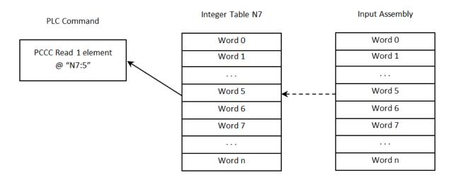
The decode ResultData begins at byte offset 16 (counting from 0) of the Input Assembly. To read the first 4 bytes of result data, issue the following PLC command:
